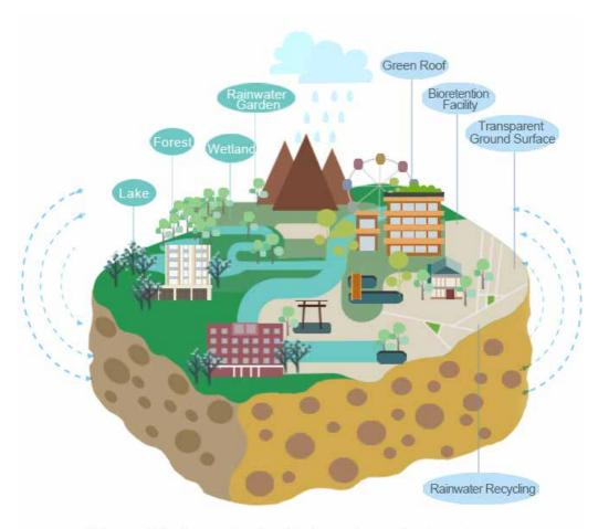
A"Sponge city" refers to a city where its urban underground water system operates like a sponge to absorb, store, leak and purify rainwater, and release it for reuse when necessary.
